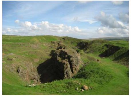
**Figure 1.** West Rigg Opencut. The quarry marks the extent of the 'limonitic' iron ore which was extracted from replacement 'flat' deposits in the Great Limestone adjacent to Slitt Vein. The vein itself, here composed mainly of quartz and a little fluorite, stands as an unworked pillar in the centre of the quarry. Narrow old lead stopes can be seen in the centre of the vein. Photo: B.Young
